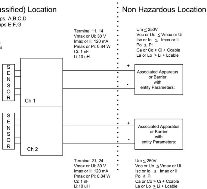
greater than the voltage ( $U_o$  or  $V_{oc}$  or  $V_t$ ) and current ( $I_o$  or  $I_{sc}$  or  $I_t$ ) and the power  $P_o$  which can be delivered by the barrier.
